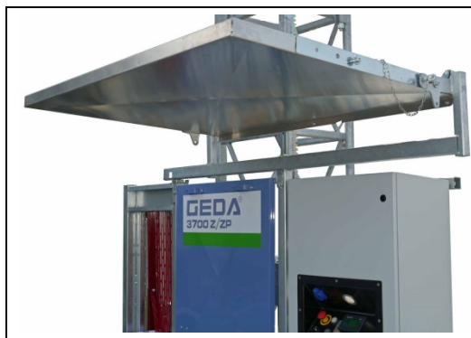
Roof, right, assembled
