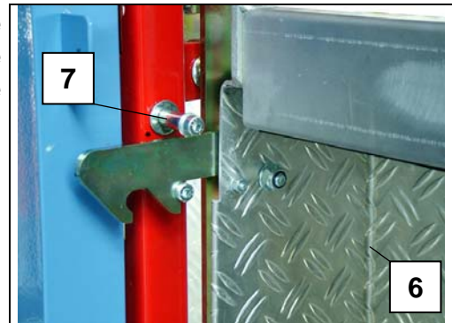
Fig. 31 Locking screw on assembly bridge
