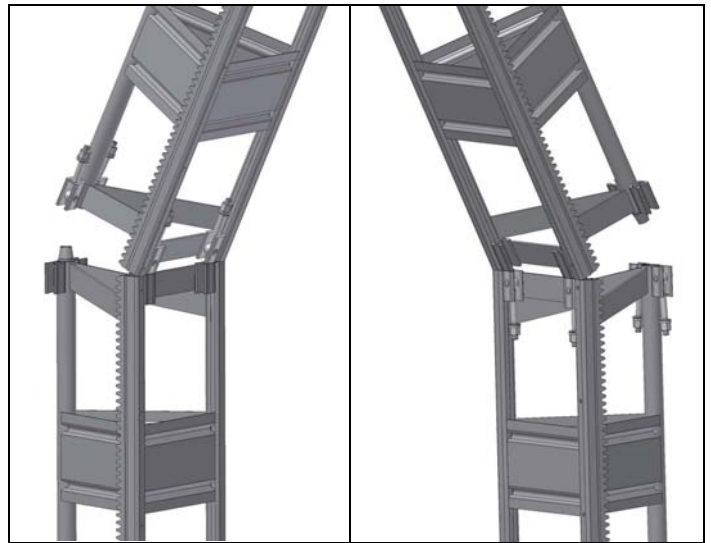
Fig. 32 Attaching the mast sections
