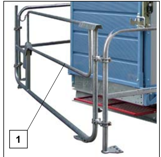
Fig. 41 Opening the barrier
