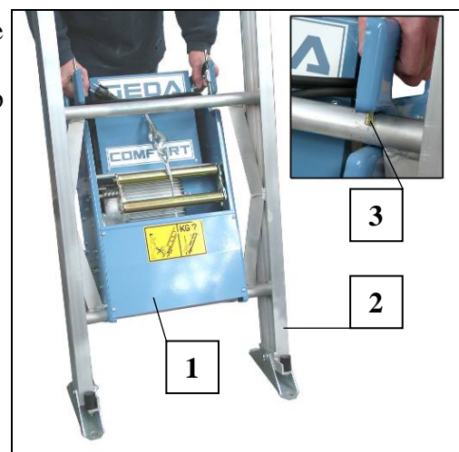
Fig. 31 Using rope winch
