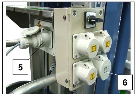
Fig. 19 Connecting the control box
