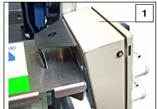
Fig. 16 Attaching the control box
