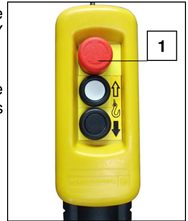
Fig. 2 EMERGENCY STOP button
