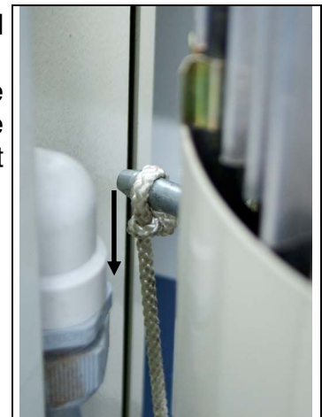
Fig. 41 Brake test pull cord
