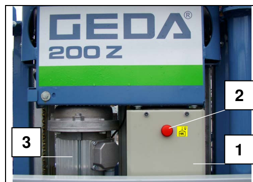
Fig. 11 Carriage switch box
