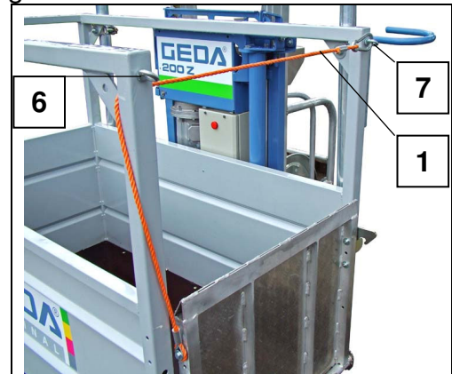
Fig. 32 Front fall protection
