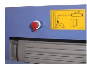
fig. 33 lubricating the tooth rack
