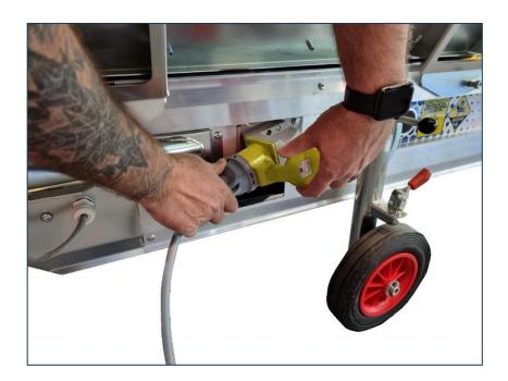
**6.** Once power is applied to the conveyor, the stop button will illuminate. The voltage indicator will also display the supply voltage. This indicates that the conveyor is ready to run.
