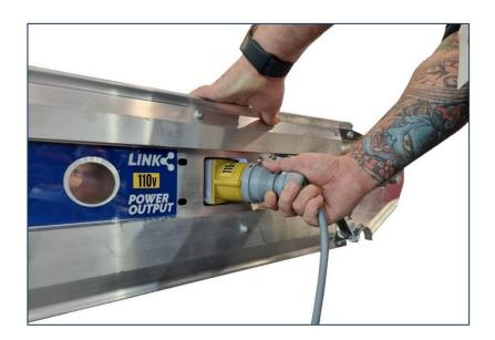
Ensure the power lead cannot get tangled in the moving belt.
