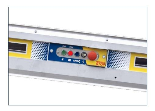
**7.** The conveyor is now ready to use. Press FWD to run the conveyor. The buzzer will sound for 2 seconds, then the belt will move. If loading with a digger or skid steer, take care not to overload the hopper.
