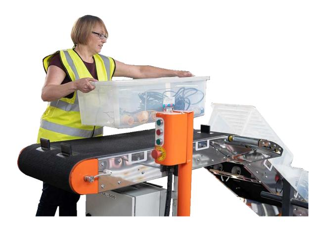
5. When the conveyor is not in use, stop conveyor belt. Ensure that no boxes or material is left on the belt.
