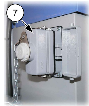
Fig. 54: Plugging in the control for special operation
