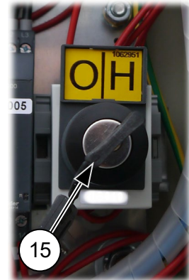
Fig. 41: Send-and-call function activated
