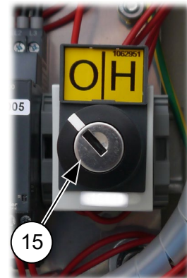
Fig. 42: Send-and-call function deactivated
