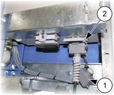
Fig. 101: Dummy plug for drop test control
