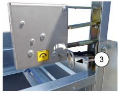
Fig. 51: Emergency release ramp/loading inside
