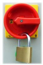
Fig. 85: Main switch secured
