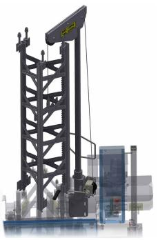
Fig. 96: Lifting, positioning of mast parts
