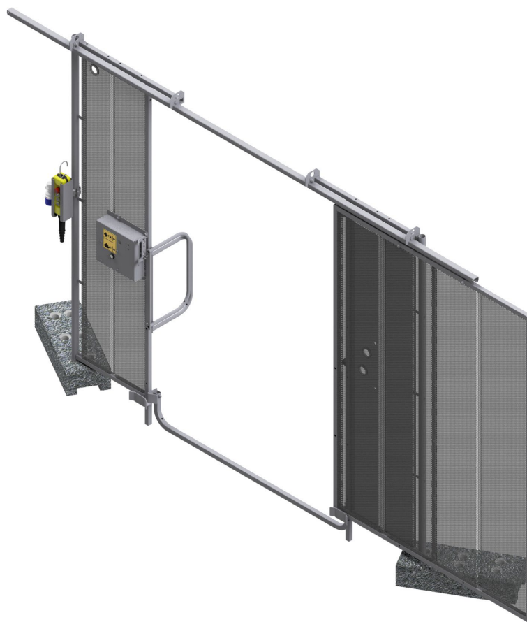
Fig. 14: Sliding door for base enclosure open
