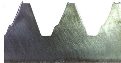
Fig. 63: Change to the contour due to wear
