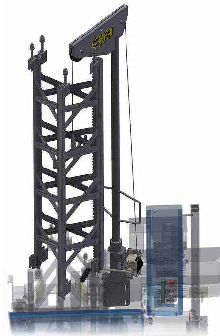
Fig. 53: Lifting, positioning of mast parts
